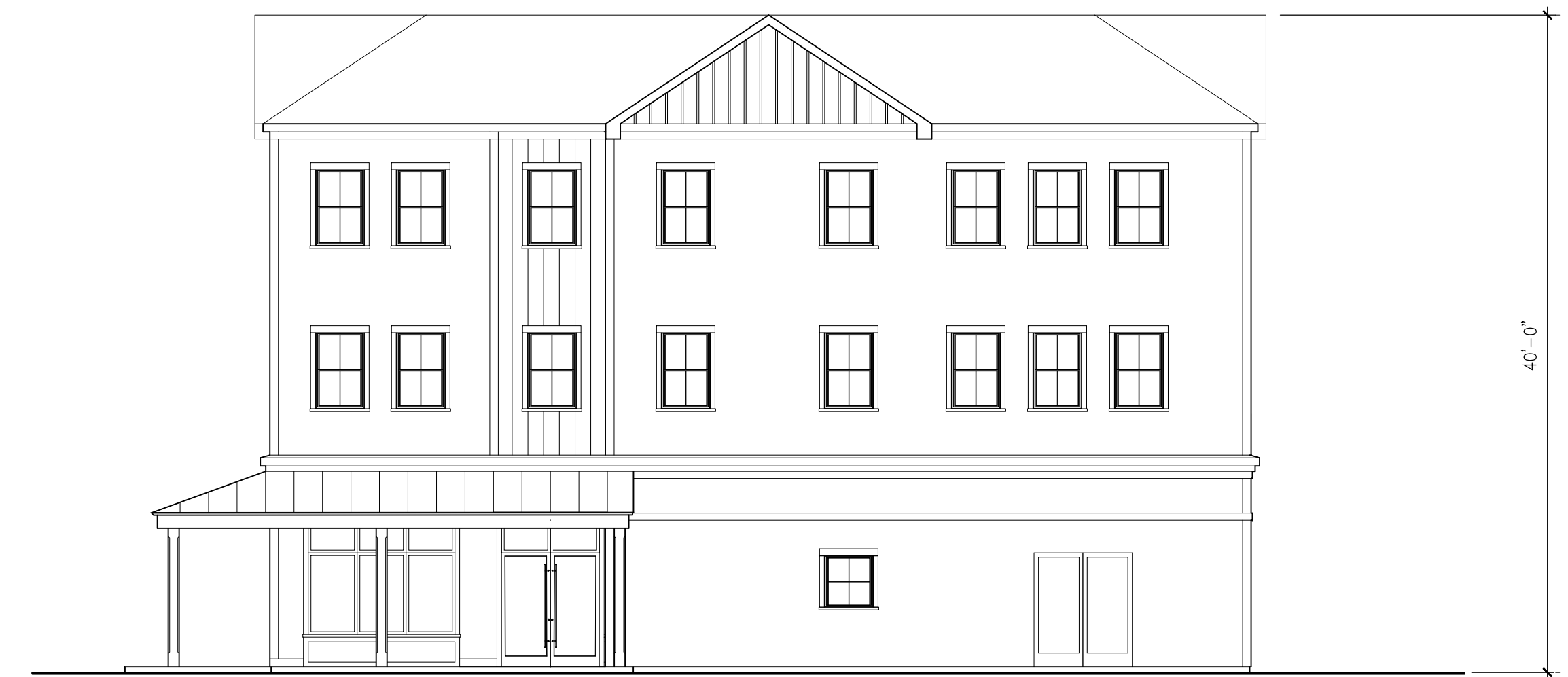
2 BUILDING A-2 - SOUTH ELEVATION SCALE: 1/8" = 1'-0"
