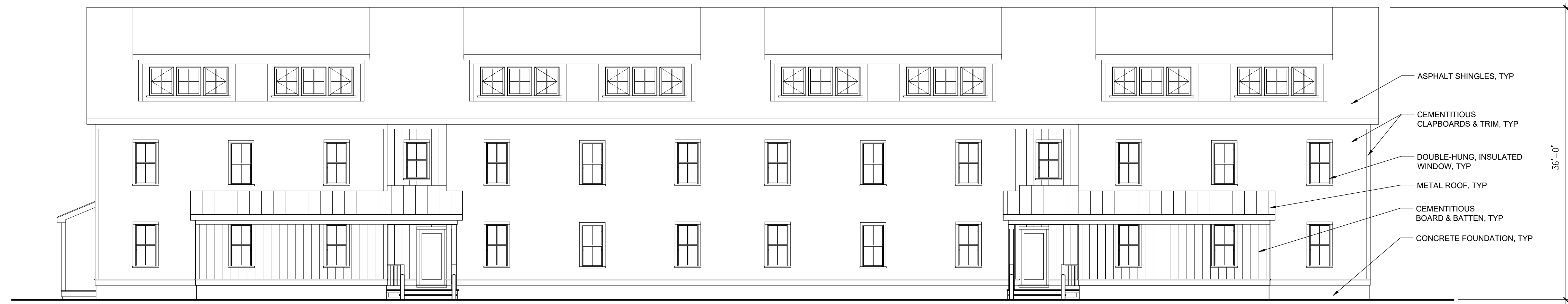
1 BUILDING B-1 - FRONT ELEVATION SCALE: 1/8" = 1'-0" (BUILDING B-2, B-3, B-4, B-5, B-6 SIM.)
