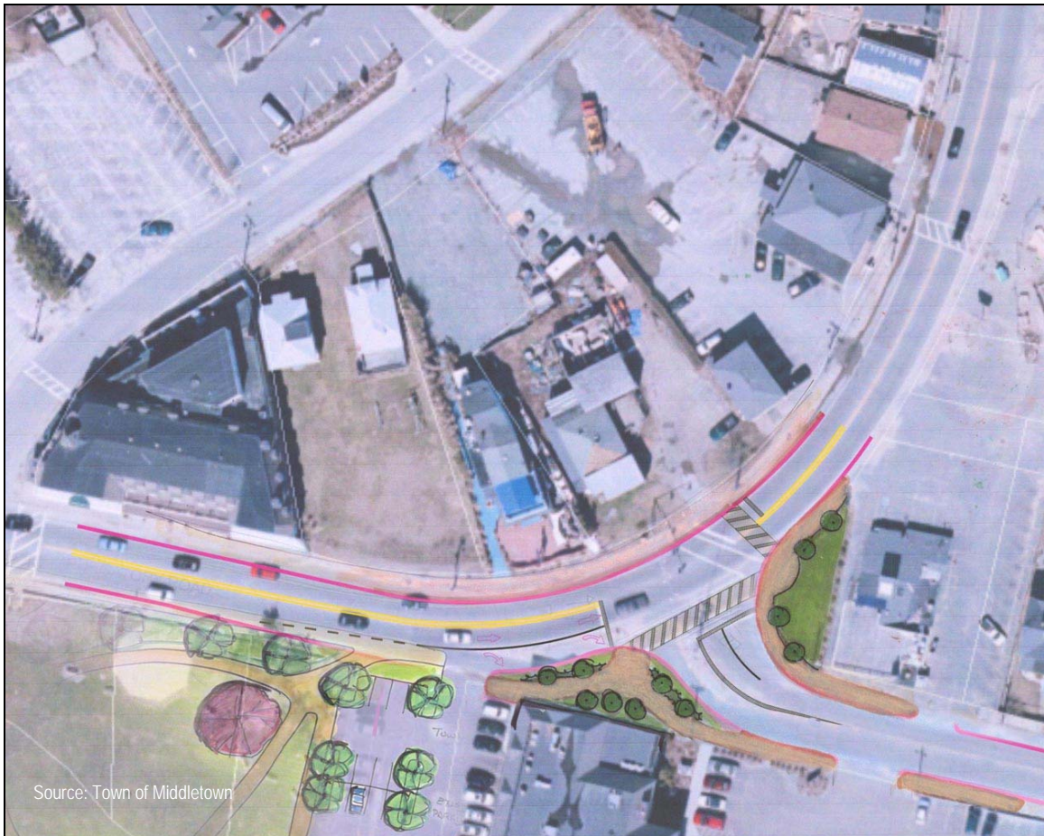
Figure 23. Conceptual illustration of bump-out at the intersection of Purgatory Road and Aquidneck Avenue.
