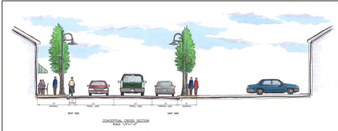
Figure 20. Conceptual typical cross section recommended for Aquidneck Avenue.
