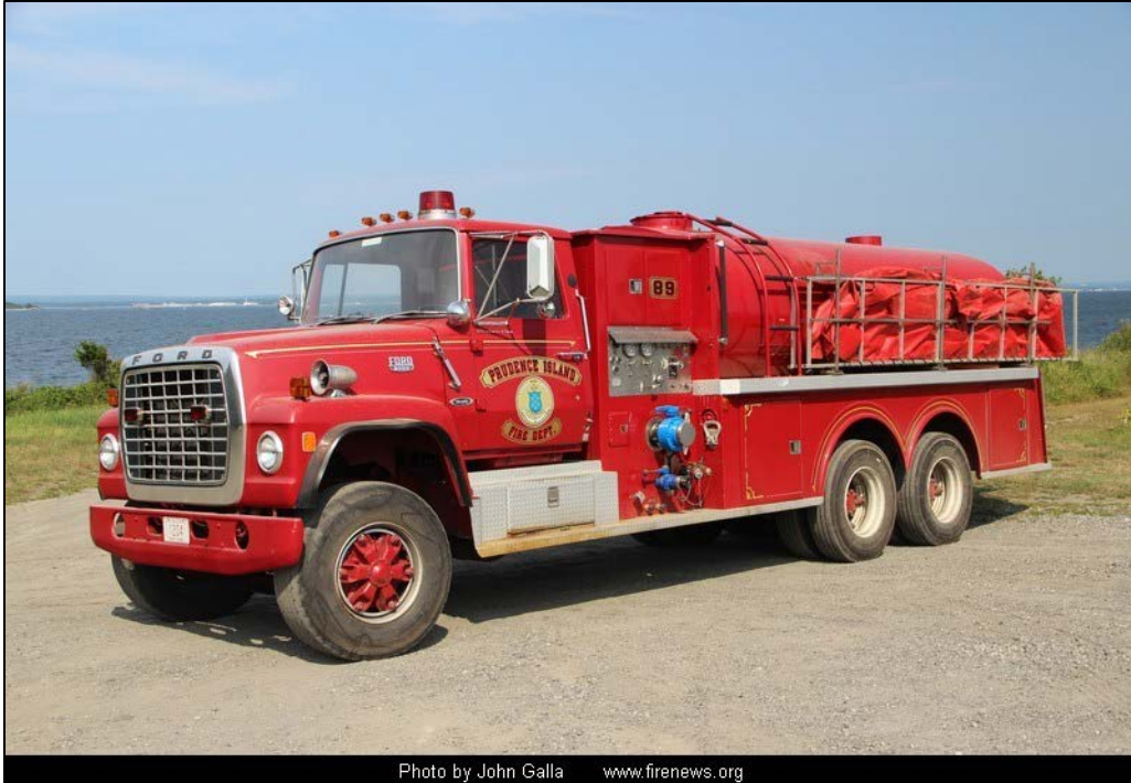
Figure 14: Tanker #1 1975 Fore/Farrar 4,000-gallon capacity
