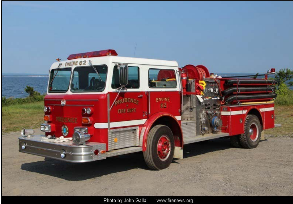
Photo by John Galla www.firenews.org Figure 12: Engine #82 1976 Maxim F 500-gallon capacity photo credit: John Galla firenews.org
