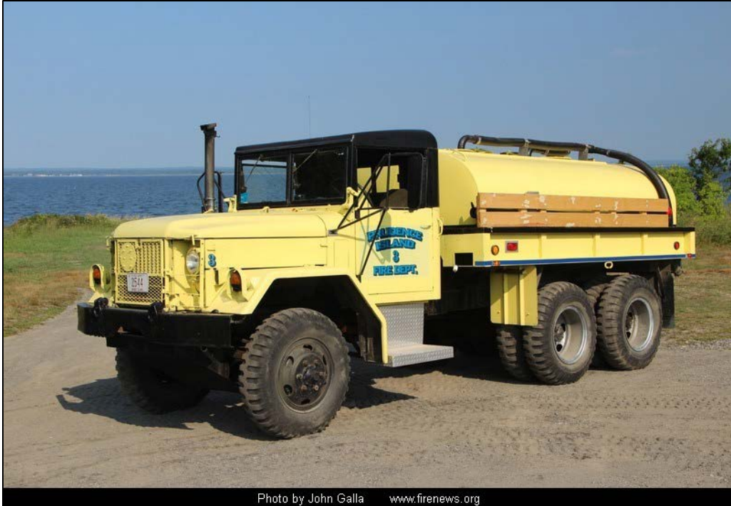
Figure 16: Tanker #3 1975 AM General 6x6 (off-road capable) 1,000-gallon capacity
