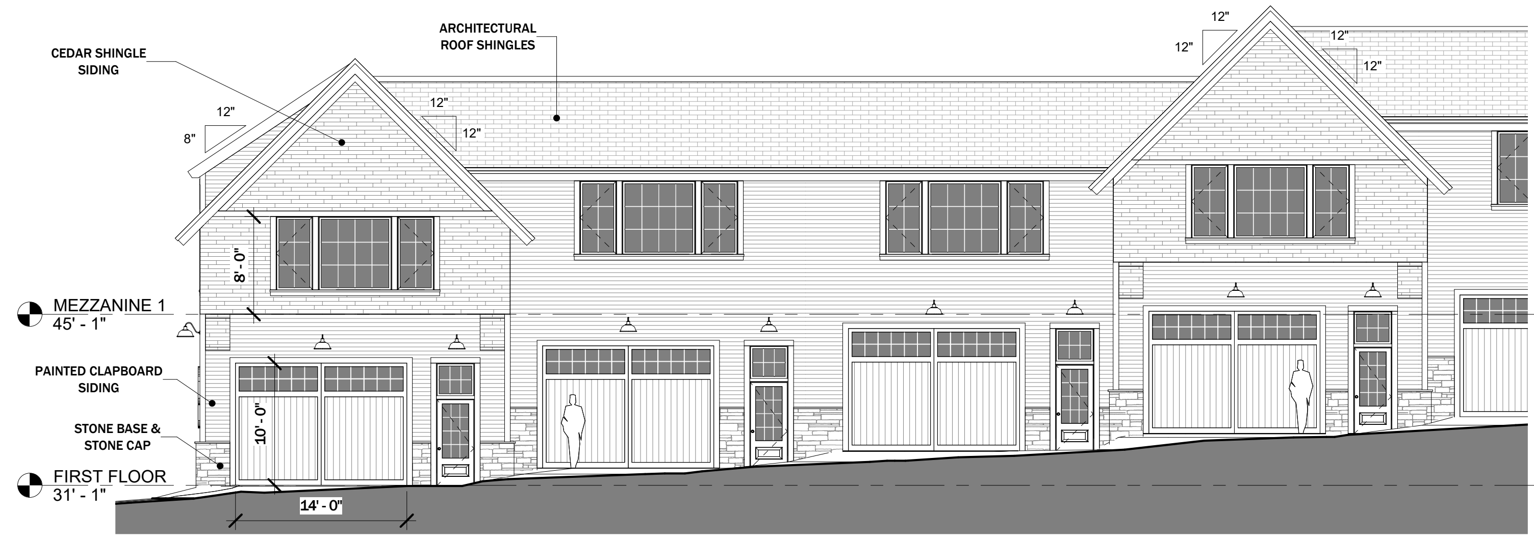
1 ENLARGED PARTIAL ELEVATION 1/8" = 1'-0"
