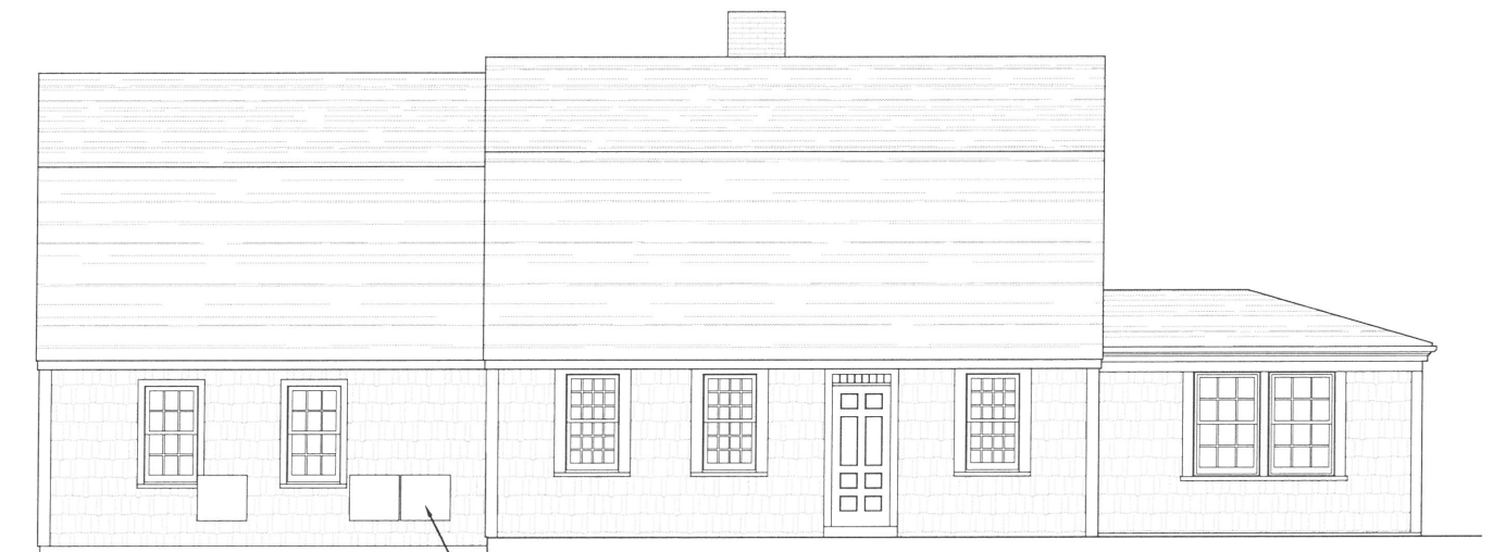
2 EAST ELEVATION - EXISTING SCALE: 1/4" = 1'-0" EXISTING WALL MTD HVAC UNITS TO BE RELOCATED
